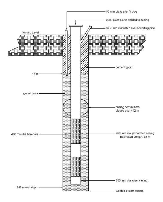
NOTE: SHOULD DRILLING OF BOREHOLE NOT BE DONE CONTINUOUSLY TO DESIRED DEPTH DUE TO UNAVOIDABLE CIRCUMSTANCES, WELL DESIGN SHALL BE CHANGED TO TELESCOPIC CASINGS 10"  $\!\!\!\!/$  X 8"  $\!\!\!\!/$
